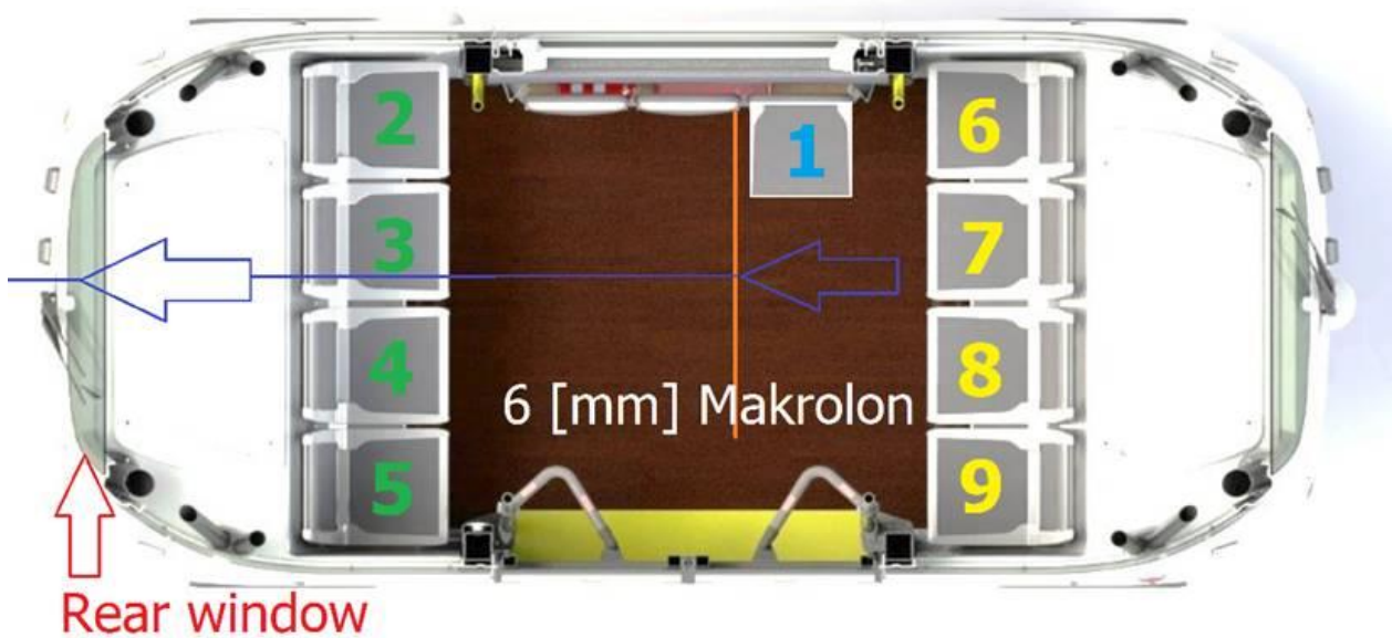
Figure 21: XA-Line Covid-19 separator window transparency testing
